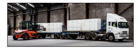
Clamp trucks should be at least 12 tonne capacity to move 3 units at once.
