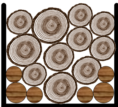
Option 2 – Front View – a few small ends facing towards centre placed against stanchions to “level” load. Where space is limited personnel can reach in and measure logs on outside edges.
