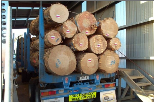
Option 2 – Front View – a few small ends facing towards centre placed against stanchions to “level” load. Where space is limited personnel can reach in and measure logs on outside edges.
