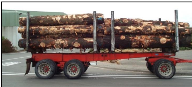
Option 2 – A few small ends facing towards centre against stanchions to “level load”
